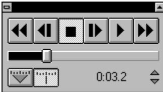
The control panel contains controls similar to those found on tape recorders. If the panel isn't visible, choose control panel from the Windows menu.
